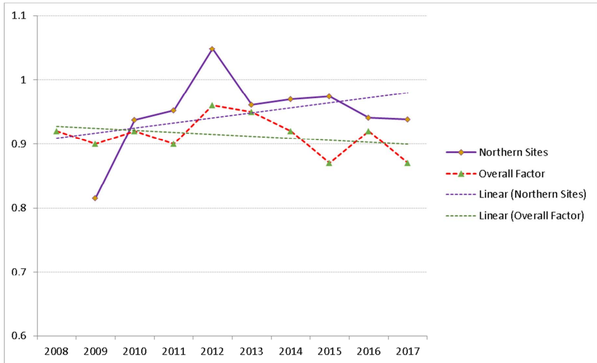
Figure 30: Calculated Overall Bias Adjustment Factor for Northern Co-Location Sites and the Overall National Factors, all for Gradko 20% TEA in Water Tubes, 2008-2017
